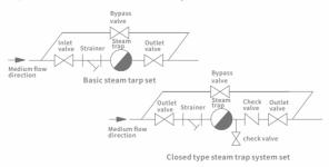
6.1 Before installing the steam trap, please check the nameplate carefully and refer to the user manual. Under the premise that the pressure, temperature, diameter, standard port, connection length, etc. are met, close the front and rear valves of the steam trap, check the flow direction of the medium and the installation direction of the product, and ensure that the arrow shown on the valve body is consistent with the flow direction of the medium.
