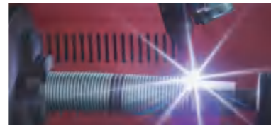
Welding of bellows assembly: microcomputer controlled welding speed to ensure the quality of the key part.
