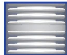
Multi-layer bellows, with guiding structure to prevent instability
