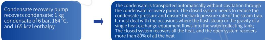
VMV condensate recovery pump (pump trap) first came from foreign technology, originally meaning "pump trap", also known as mechanical power pump. It uses the principle of steam trap and relies on steam, air and other gases as power to transport condensate from low-pressure area to high-pressure area, or from negative pressure area (vacuum) to normal pressure area.
