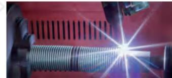
Welding of bellows components: Microcomputer controls the welding speed to ensure the quality of critical components
