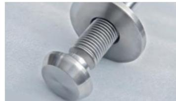
Conical sealing: No impurities remain on the sealing surface. When it tends to close, the sealing surface has a self-cleaning effect to achieve linear sealing.
